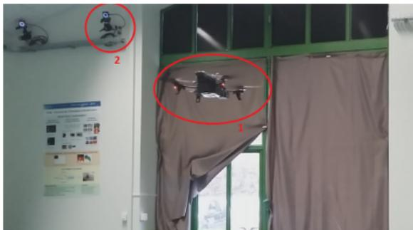
FIGURE – 1. Parrot AR.Drone 2.0. 2. Motion capture system.
